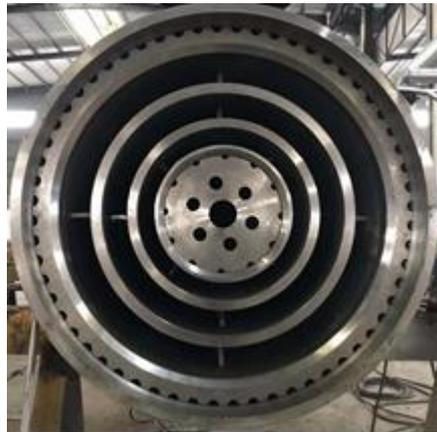
**Figure 3.** Head diagram of five-channel vortex flow low-NO<sub>x</sub> burner.
