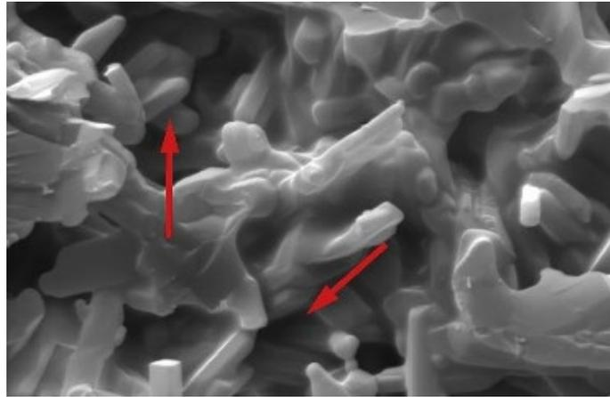
**Figure 2.** SEM image of fracture surface of SiC sample added
