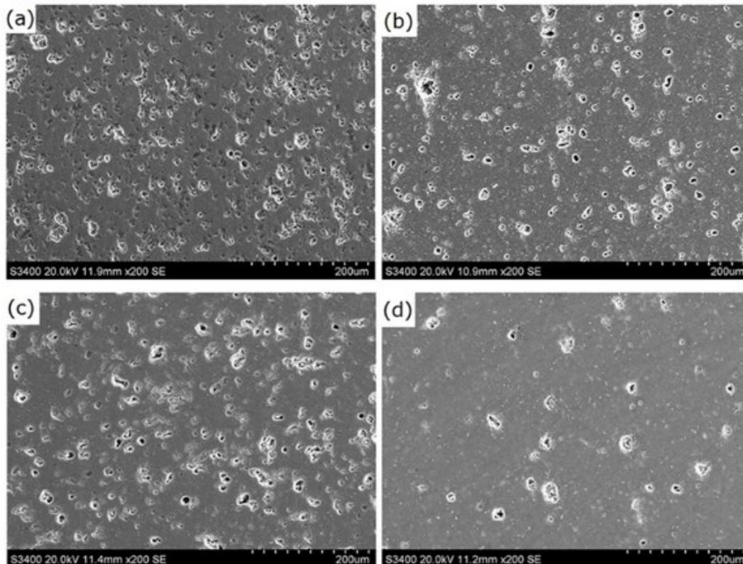
**Figure 4.** Surface morphology of samples prepared by adding 30 wt% SiC at different sintering temperatures: (a)  $1250^\circ C$ , (b)  $1300^\circ C$ , (c)  $1350^\circ C$  and (d)  $1400^\circ C$ .
