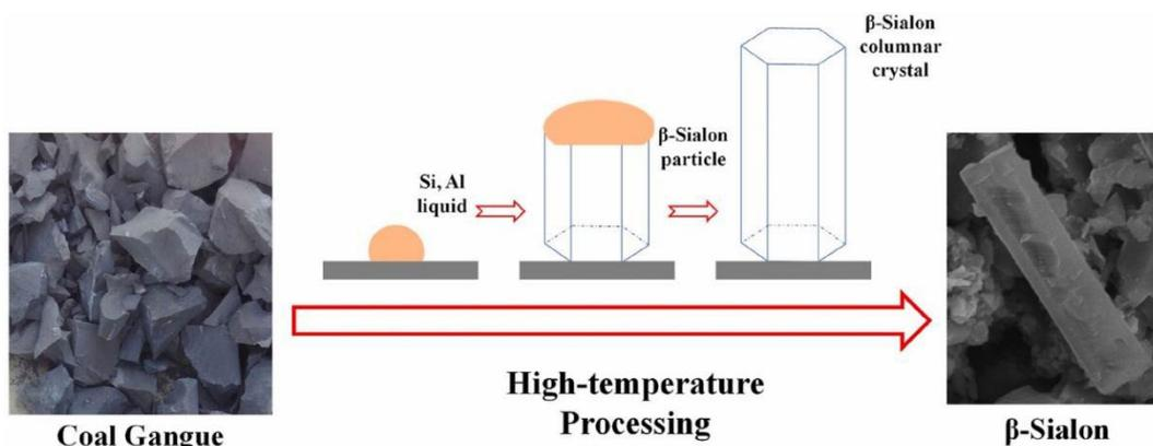
**Figure 3.** The reaction process of transforming coal gangue into β-SiAlON phase.
