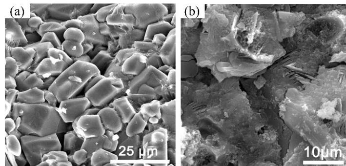
**Figure 5.** SEM images of desert sand cement clinker and hydration product: (a) clinker, (b) hydration product.
