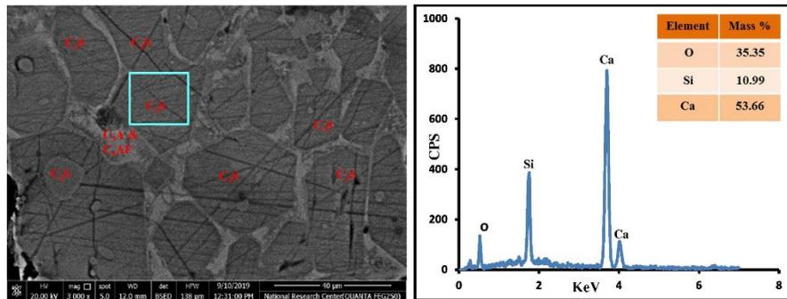
**Figure 4.** SEM images of basalt cement clinker.
