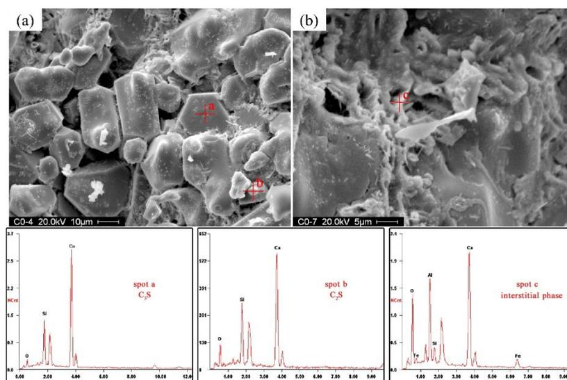
**Figure 1.** SEM images of iron tailings cement clinker: (a)  $\text{C}_3\text{S}$  and  $\text{C}_2\text{S}$ , (b) interstitial phase.
