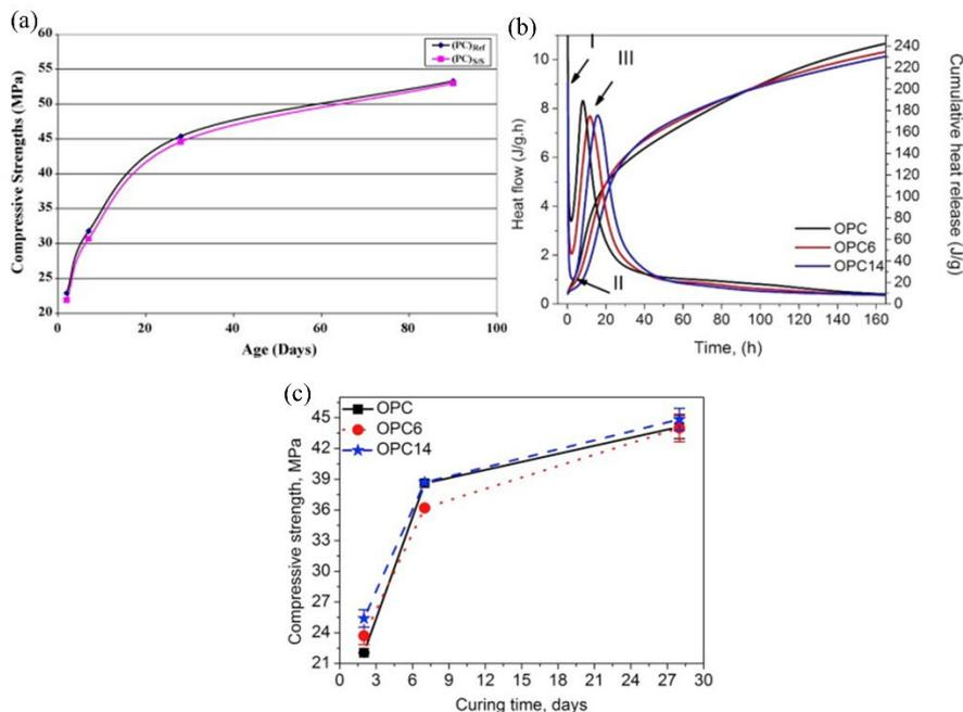
**Figure 2.** Compressive strength and hydration heat of steel slag-based cement: (a) compressive strength of cement with steel slag, (b) hydration heat of cement with ladle metallurgy stainless steel slag, (c) compressive strength of cement with ladle metallurgy stainless steel slag.
