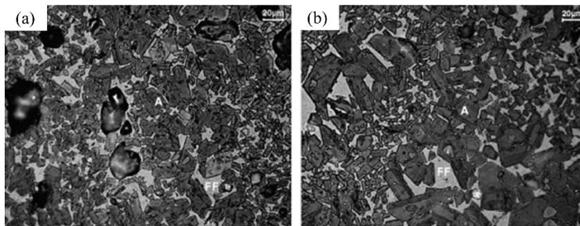
**Figure 3.** SEM images of ceramic waste cement clinker: (a) reference sample, (b) ceramic waste cement clinker. (A: C<sub>3</sub>S, FF: interstitial phase).
